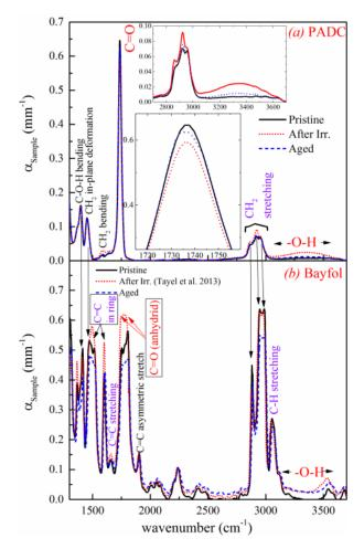
Figure (7): Infrared absorption spectra for pristine sample, sample irradiated with 1 MGy dose, and sample irradiated with 1 MGy dose and aged for 7 years. Material represented in part (*a*) is polyallyl diglycol carbonate and in part (*b*) is Bayfol CR
