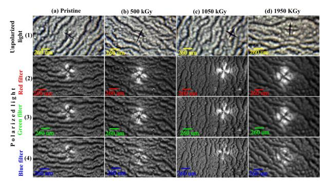
Figure 3: Polarized and unpolarized light optical microscope images for Bayfol samples at different doses. The scale bar may change within 5%.
