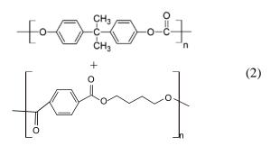
Bayfol is manufactured by Bayer (Leverkusen, Germany), specimen size was 1 cm  $\times$  1 cm with an average thickness of 375  $\mu$  m and density 1.23 g/cm<sup>3</sup>. The two materials represent the morphological structure of considerable fraction of biological tissues and industrial materials.
