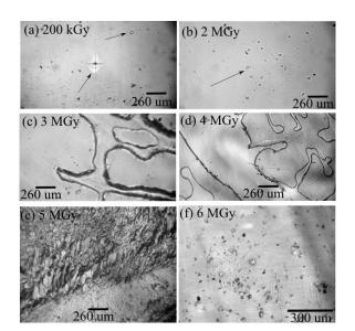
Figure (1): Optical microscope image of resin extension on the surface of PADC samples at different doses. The embryo of the resin begins to appear at doses of 200 kGy and spread out through the surface of the samples as the dose increase. At 6 MGy dose, the resin covers most of the surface of the sample. The scale bar may vary within 5% due to the auto-focus function of the CMOS CCD camera.
