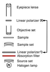
Figure (2): Modified setup for the polarized light measurements. Imaging was performed without and with absorption filters; with Red ( $\lambda = 600$  nm), Green ( $\lambda = 555$  nm), and Blue ( $\lambda = 420$  nm)
