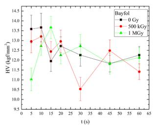
Figure (5): Indention time-dependent micro-hardness values of Bayfol for samples irradiated with different doses.
