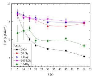
Figure (4): Indention time-dependent micro-hardness values of PADC for samples irradiated with different doses
