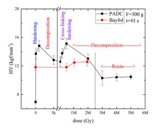
Figure (6): The variation of HV with dose for PADC and Bayfol nuclear track detectors.
