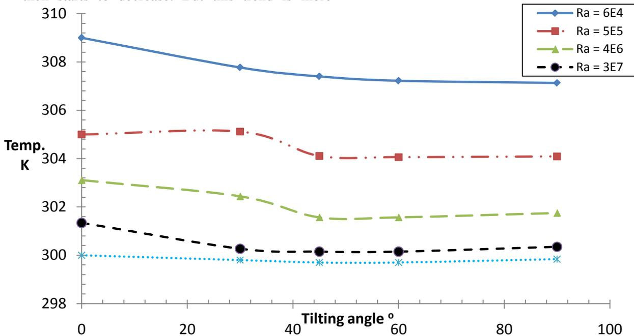
Fig. 10 Variation of average surface temperature with tilting angle at different Ra
