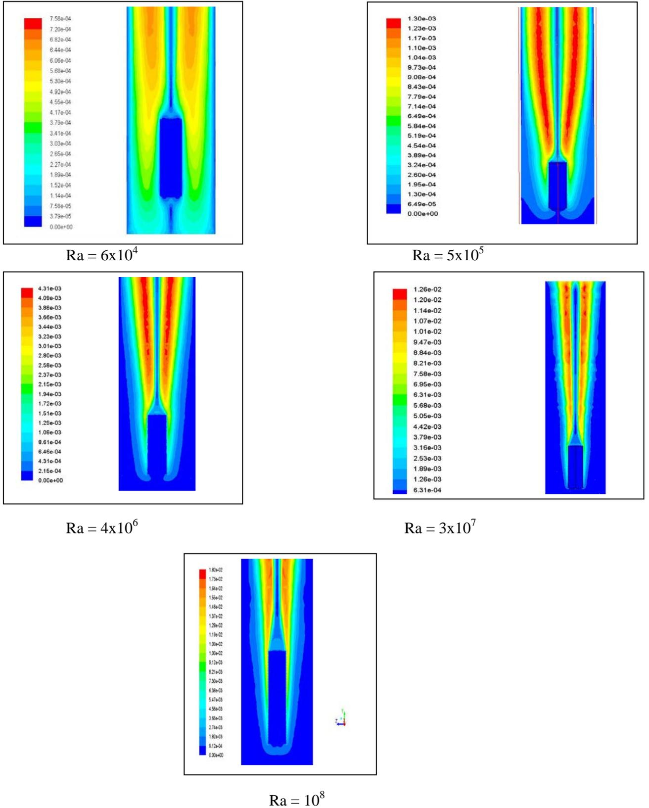
**Fig. (4): Velocity contours at various  $Ra$  for the case of vertical position**
