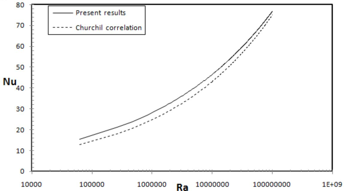
**Fig. (2): Variation of the average Nu with Ra for the case of vertical cylinder**
