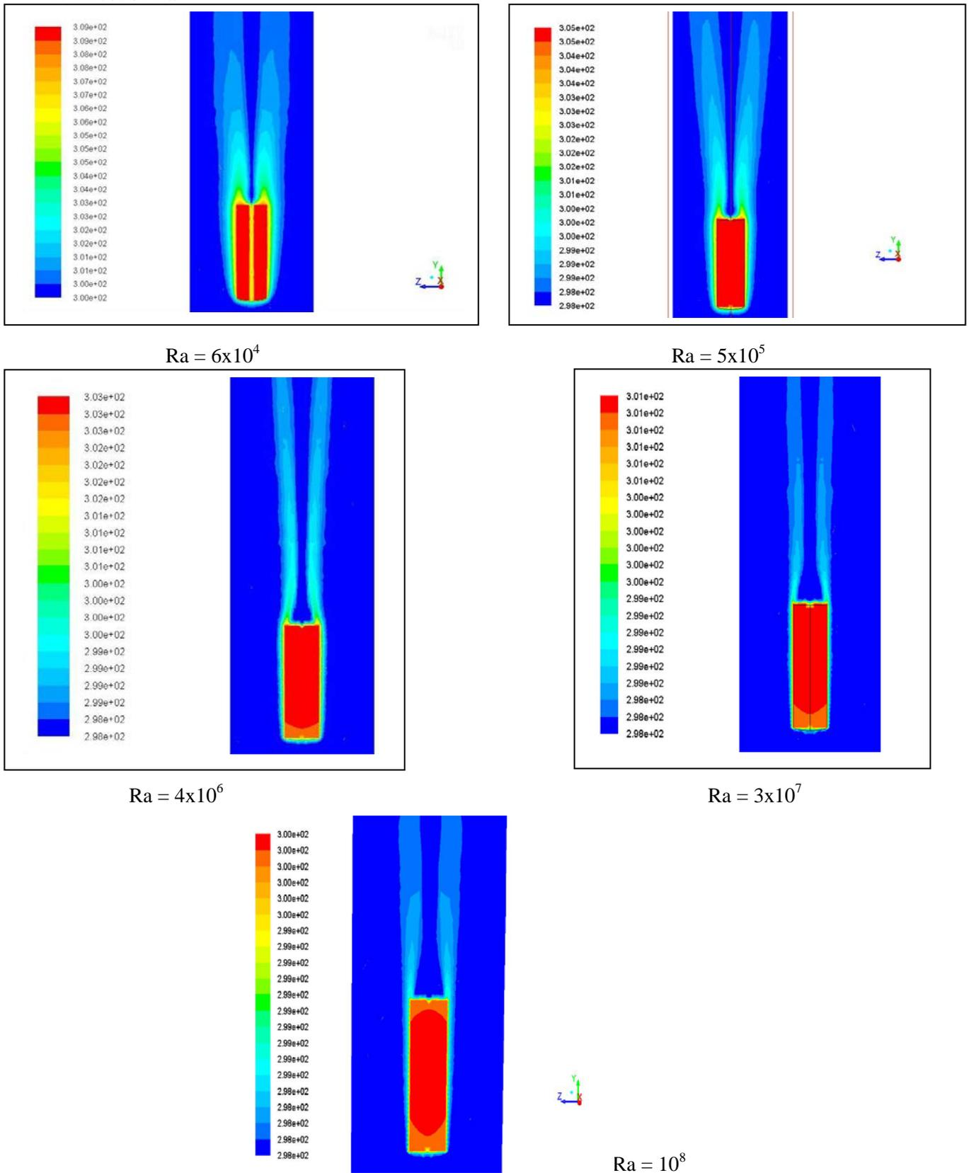
**Fig. (3): Temperature contours at various Ra for the case of vertical position**
