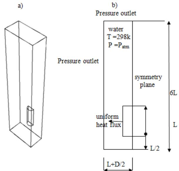
Fig.(1):a) 3D view of cylinder suspended in stagnant water
