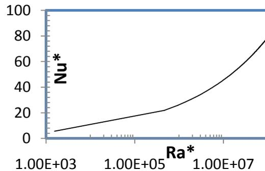
Fig.11 Best fit curve for Nu\* with Ra\*at any tilting angle°.
