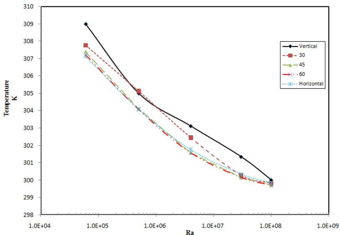
Fig. (6) Variation of average surface temperature with Ra at different tilting angles
