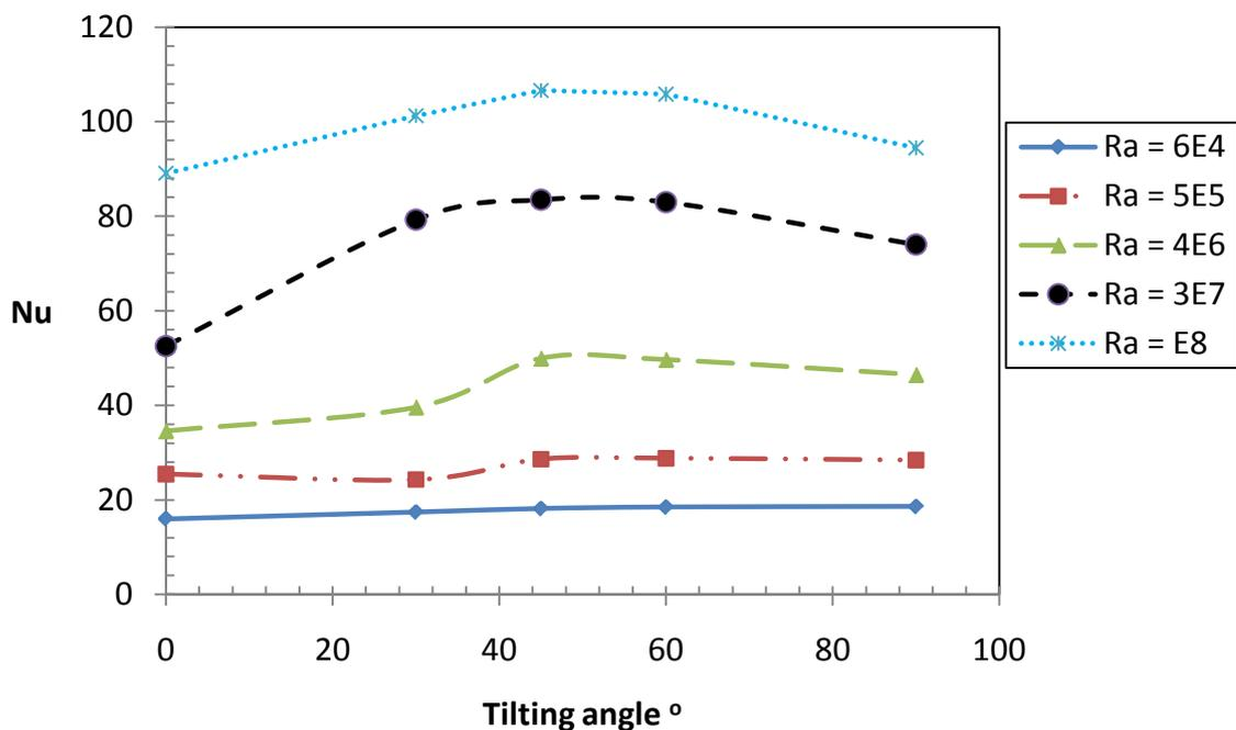
Fig. (9) Variation of Nu with tilting angles at different Ra
