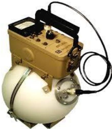
Figure (6): ESP-1 neutron detector
