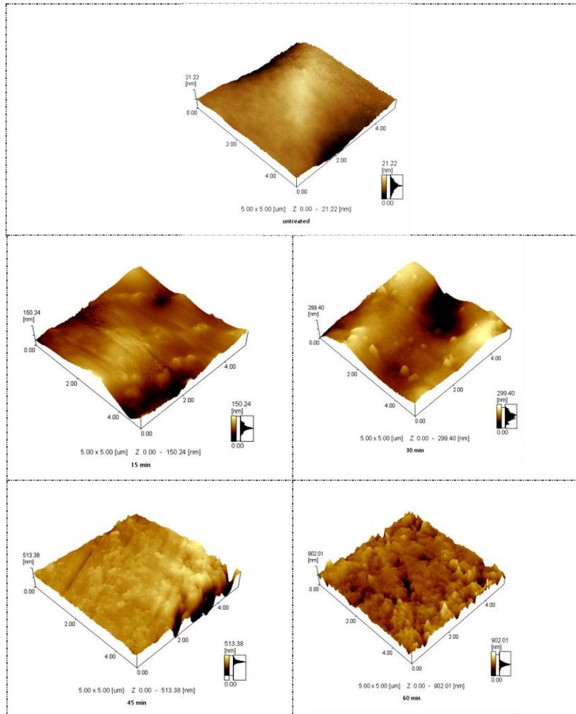
Figure (2): AFM images for untreated and plasma treated samples for different treatment time
