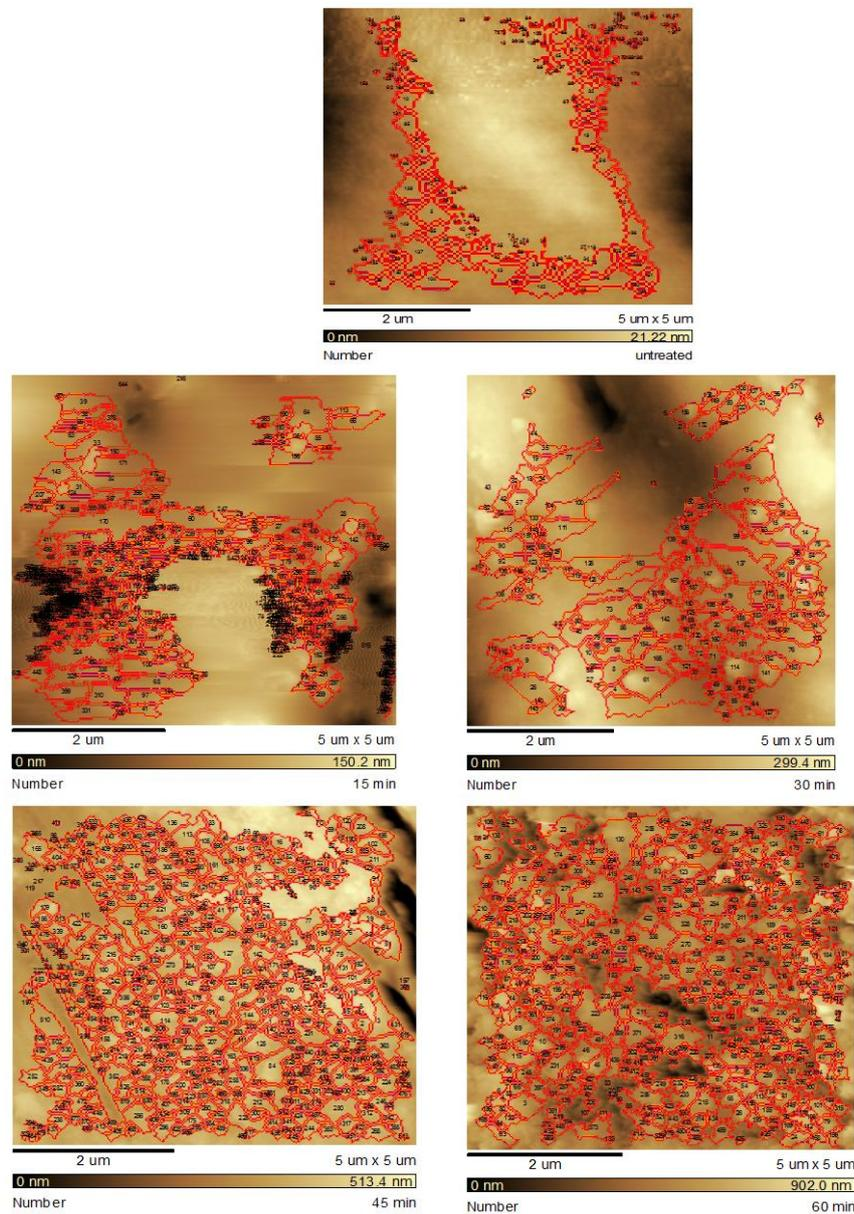
**Figure (3): AFM particle analysis for untreated and plasma treated samples for different treatment time**
