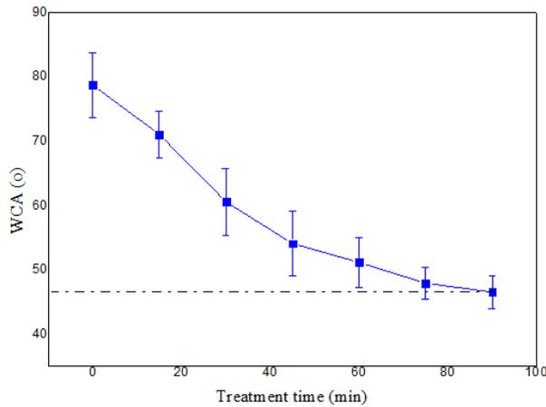
Figure (4): Water contact angle as a function of plasma treatment time
