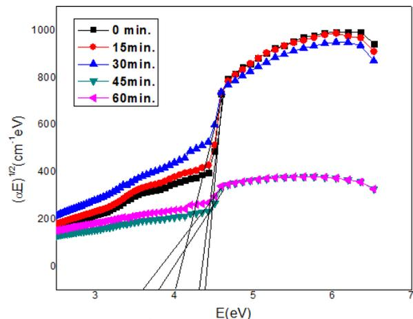
Figure (6):  $(\alpha h\nu)^{1/2}$  as a function of photon energy for unirradiated and O<sub>2</sub> plasma irradiated Cu/PMMA nanocomposite films
