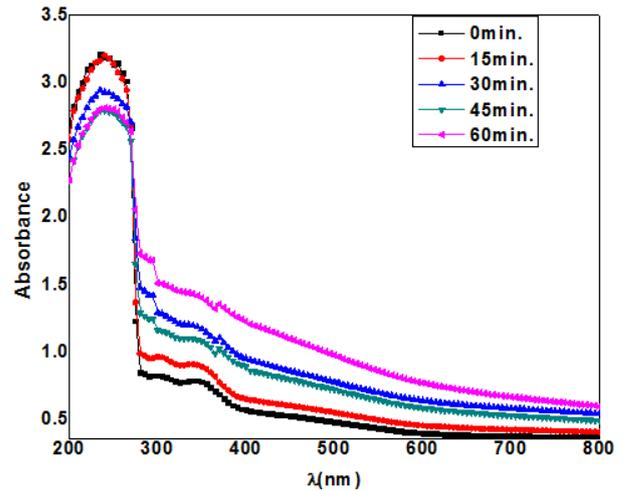
Figure (5): UV-vis absorption spectra of Cu/PMMA nanocomposite samples treated with O<sub>2</sub> plasma for different irradiation times
