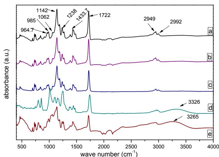
**Figure (1): FTIR spectra of untreated [a] and treated films for 15 min [b], 30 min [c],**
