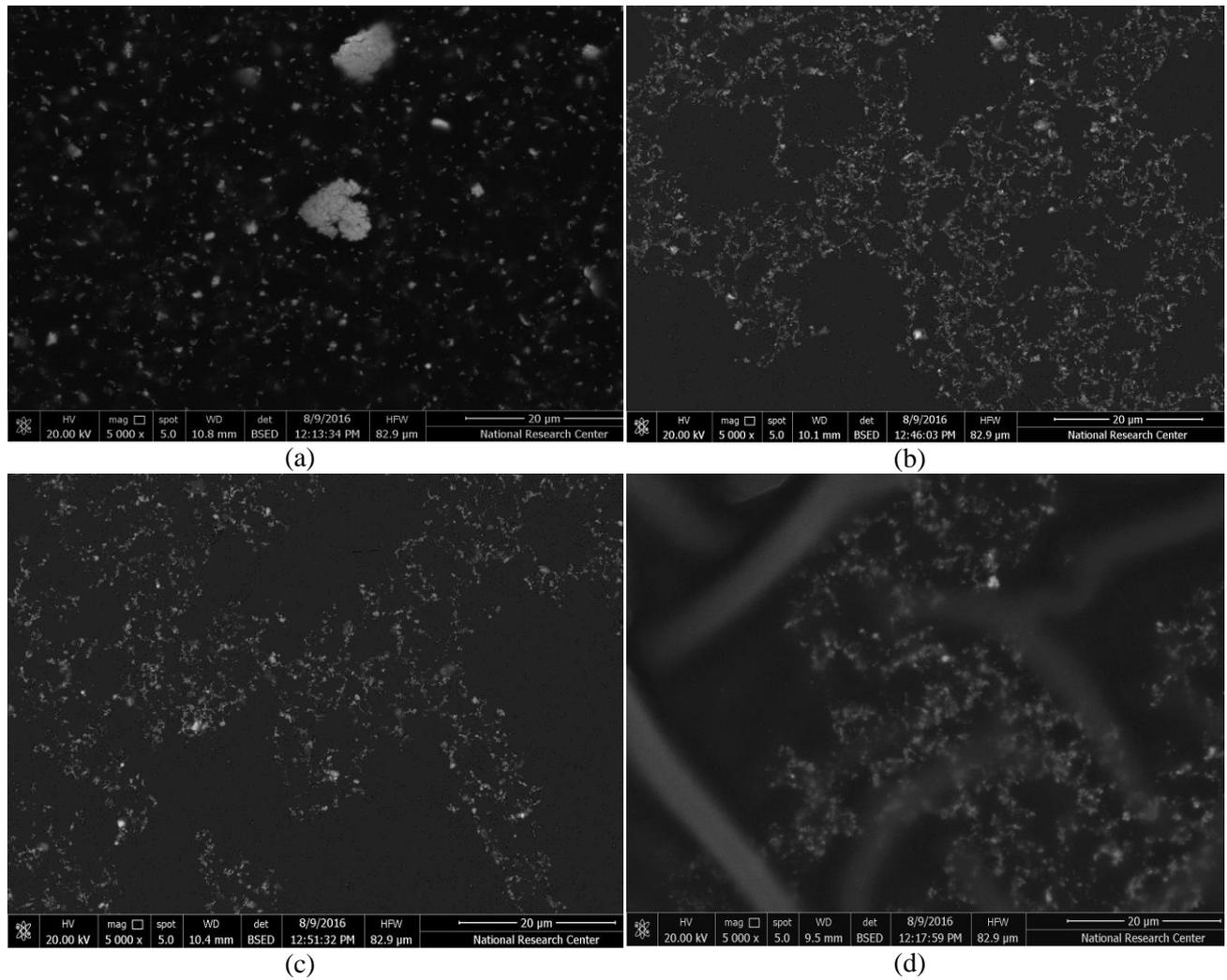
**Fig. (2): SEM for (a) untreated Cu/PS (1 Wt. %) composite sample and plasma treated samples for different exposure time durations: (b) 15 min, (c) 30 min, (d) 60 min**
