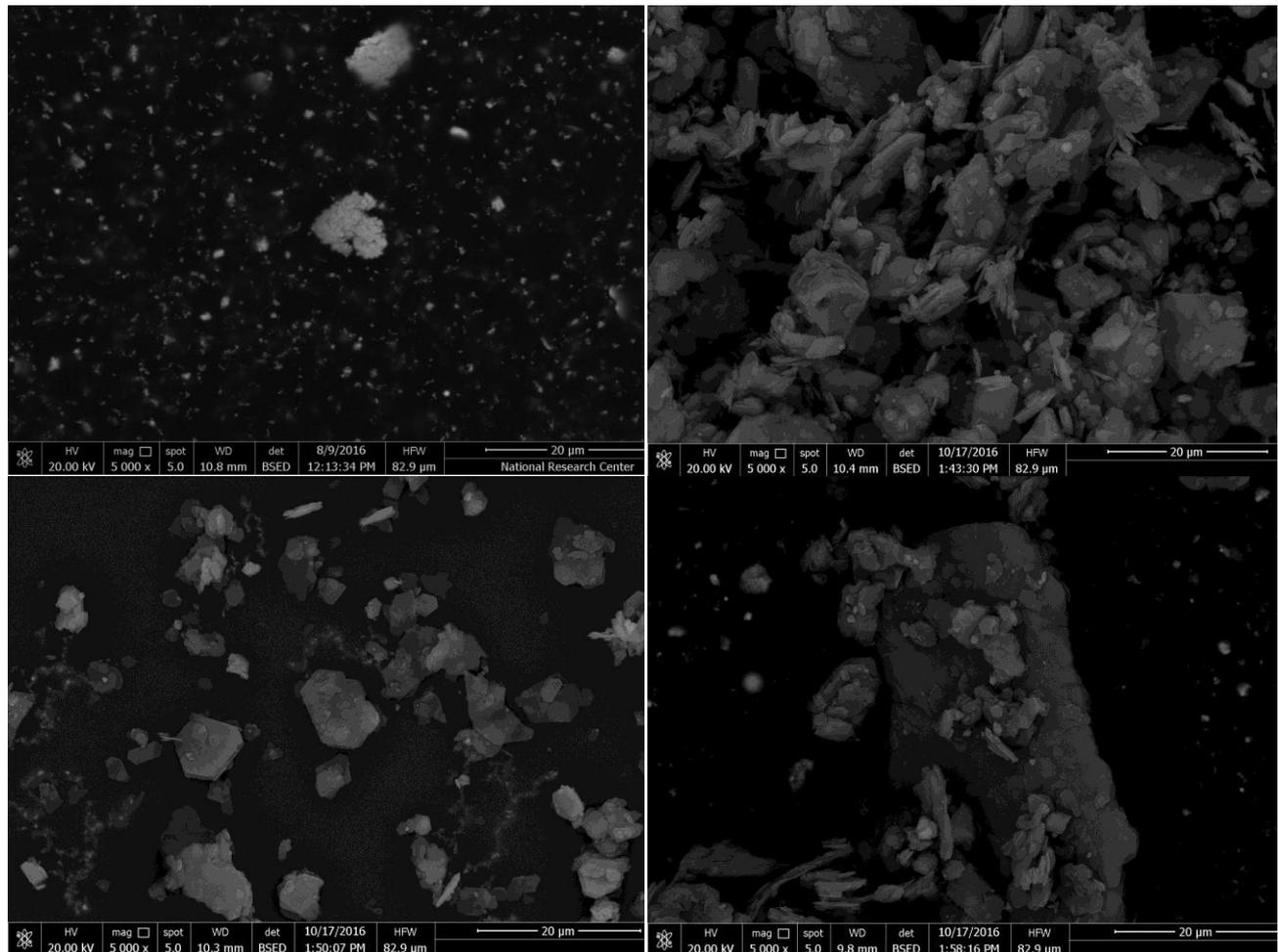
**Fig. (3): SEM for (a) untreated Cu/PS (1 Wt %) composite sample and gamma treated samples for different radiation doses: (b)10 KGy, (c) 30 KGy , (d) 50 KGy**
