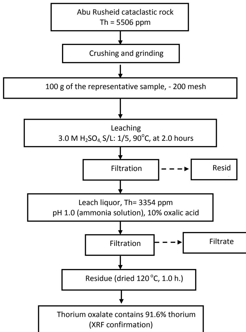
Fig. (7): Proposed flow sheet for leaching thorium with 3.0 M H<sub>2</sub>SO<sub>4</sub> from the representative samples (cataclastic rocks), Abu Rusheid area, south Eastern Desert, Egypt
