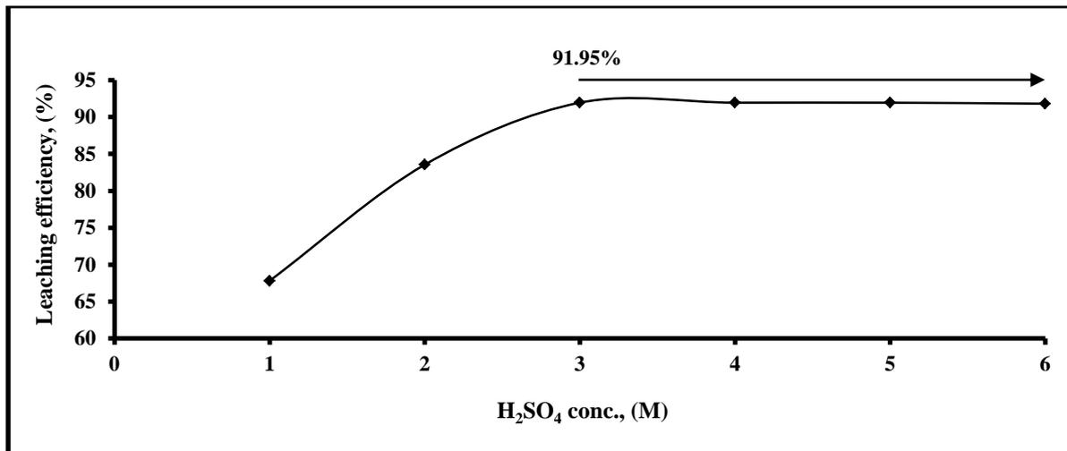
**Fig. (2): Effect of H<sub>2</sub>SO<sub>4</sub> concentration on thorium leaching efficiency (%)**
