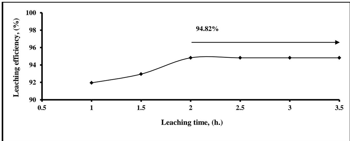
Fig. (4): Effect of leaching time on thorium leaching efficiency (%)
