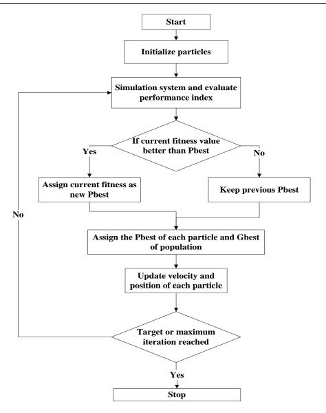
Figure (3): Flowchart of the presented PSO technique controller
