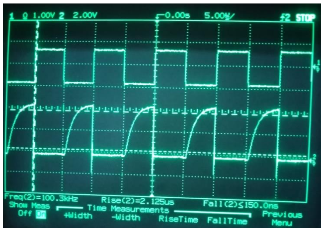
Fig. (14): Sample of measured output pulse (down) with reference input pulse (up) using a digital oscilloscope first group device one after 3.0 Gy gamma irradiation.
