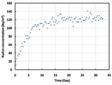
Figure (11) Radon concentration inside the radon calibration system at Najran University, Saudi Arabia
