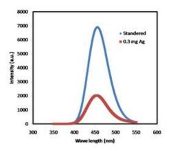
Figure (7): Luminescence spectra of the prepared ZnS: Ag, Cl and the stander sample
