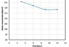
Figure (12): Radon concentration inside the radon calibration system measured with local CPRD cell
