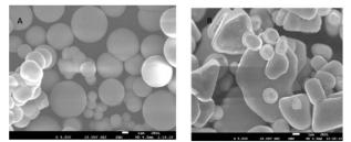
Figure (2): The SEM image of (A) prepared sample, and (B) stander sample
