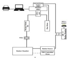
Figure (10): Radon calibration system with dual radon monitor
