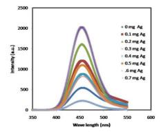
Figure (5): Luminescence spectra of ZnS: Ag, Cl measured at the different concentration of AgNO3
