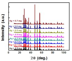
Figure (4): The XRD patterns of pristine and activated ZnS samples
