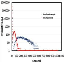
Figure (9): The pulse height spectra of 241Am  $\alpha$ -particles and 60KeV  $\gamma$  Rays measured by using standered and prepared samples (ZnS; Ag) without firing
