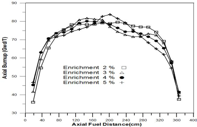
Fig. (5): Fuel Burnup (Gwd/T) versus axial fuel distance (cm)
