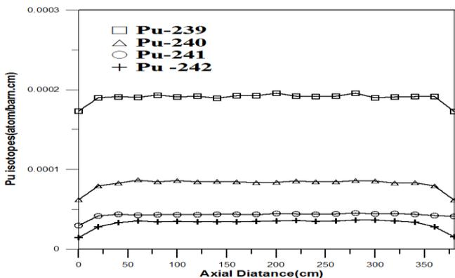
Fig. (7): Pu isotopes versus Axial core distance (cm) for 4 % Enrichment at discharge burnup 60 Gwd/T and 5 year cooling.
