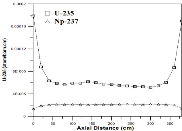
Fig. (6): U-235 and Np-237 versus Axial core distance (cm) for 4 % Enrichment at discharge burnup 60 Gwd/T and 5 year cooling.
