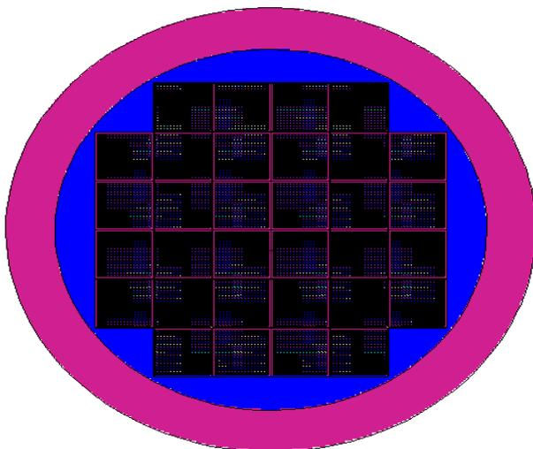
Fig. (3): MCNPX cross sectional view of GBC-32 cask model
