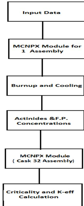
Fig. (4): Computational Procedure of The Model
