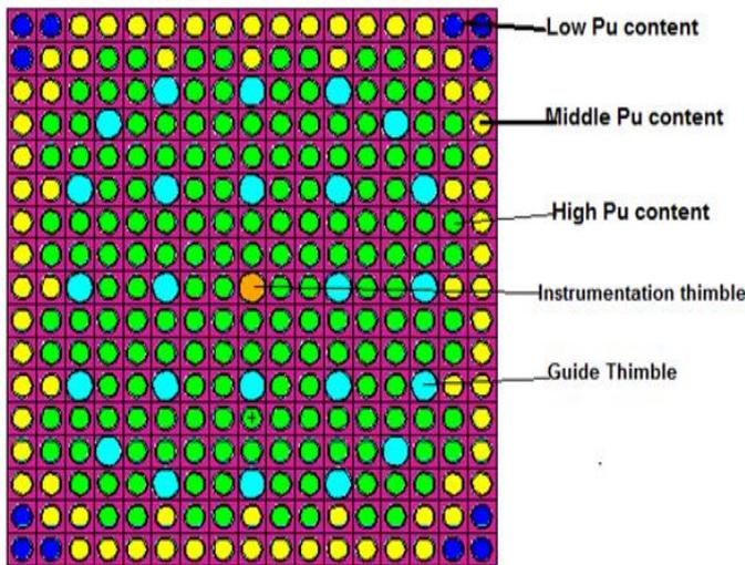
Fig. (2):MCNPX Horizontal Cross section of MOX assembly Model
