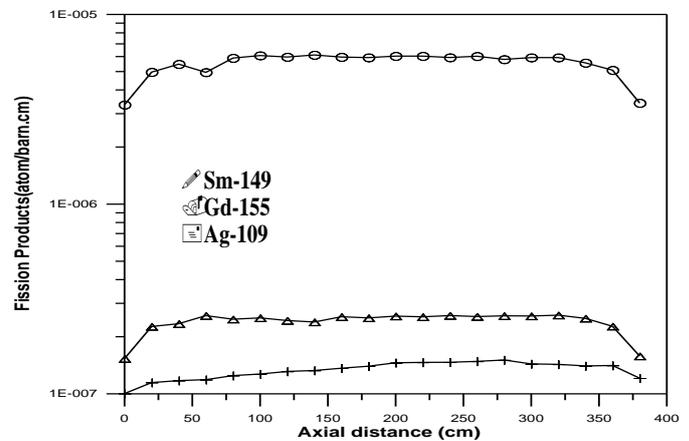
Fig. (9): Fission product versus Axial core distance (cm) for 4 % Enrichment at discharge burnup 60 Gwd/T and 5 year cooling.
