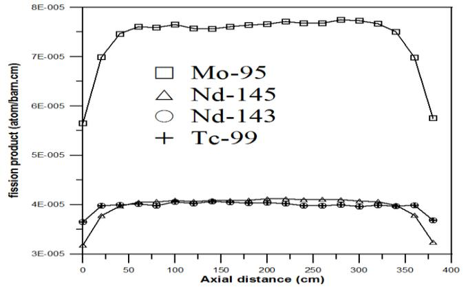
Fig. (8): Fission product versus Axial core distance (cm) for 4 % Enrichment at discharge burnup 60 Gwd/T and 5 year cooling.
