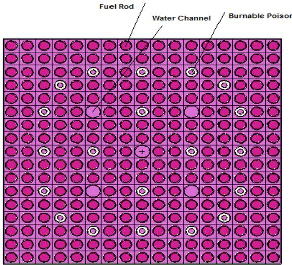
Fig. (1): MCNPX model for PWR- UO<sub>2</sub> Assembly Model
