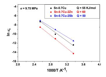
Fig. (11): Linear relationships of the strain rate-temperature of Sn-0.7 Cu, Sn-0.7 Cu-2Z n and Sn-0.7 Cu-2S b alloys crept at 9.8 MPa
