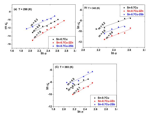
Fig. (10): The relation between ln  $\epsilon_s$  against ln  $\sigma$  for Sn-0.7 Cu, Sn-0.7 Cu-2Z n and Sn-0.7 Cu-2Sb alloys at (a) 298 K, (b) 343 K and (c) 393 K
