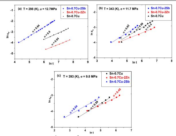
Fig. (8): Shows the relations between  $\ln \varepsilon_{tr}$  against  $\ln t$  for Sn-0.7 Cu, Sn-0.7 Cu-2Zn and Sn-0.7 Cu-2Sb alloys tested at (a) 298K, (b) 343K and (c) 393K
