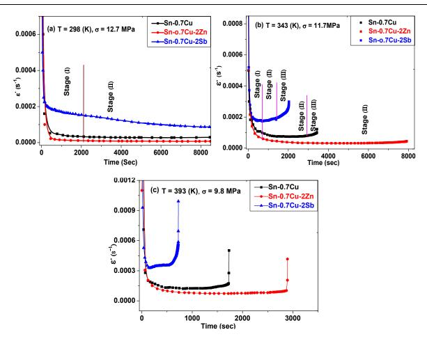
Fig. (7): shows strain rate - time relationships at a) 298 K, 12.7 MPa, (b) 343K, 11.7 MPa and (c) 393 K, 9.8 MPa for Sn-0.7 Cu, Sn-0.7Cu-2.0 Zn and Sn-0.7 Cu-2.0Sb solders
