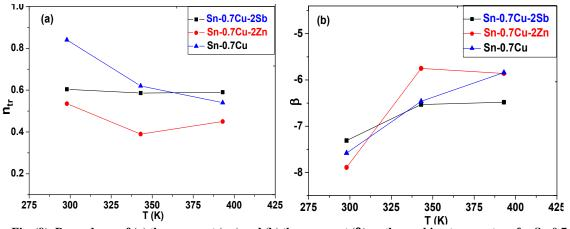
Fig. (9): Dependence of (a) the exponent  $(n_{tr})$  and (b) the exponent  $(\beta)$  on the working temperature for Sn-0.7 Cu, Sn-0.7 Cu-2 Zn and Sn-0.7 Cu-2Sb alloys
