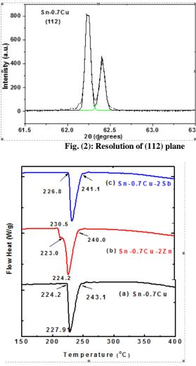
Fig. (3): DSC curves of (a) Sn-0.7Cu (b) Sn-0.7Cu-2.0Zn (c) Sn-0.7Cu-2.0Sb solder
