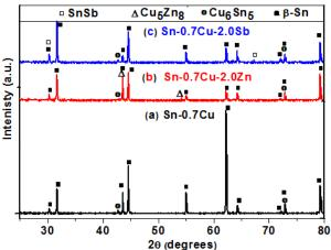
Fig. (1): X-Ray Diffraction of (a) Sn-0.7Cu, (b) Sn-0.7Cu-2.0Zn and (c) Sn-0.7Cu-2.0Sb lead free solder alloys
