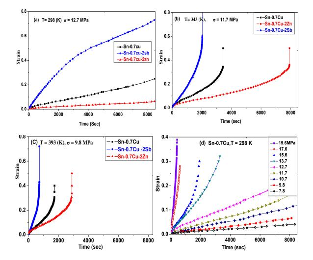
Fig. (6): Shows the creep behavior at (a) 298K, 12.7 MPa, (b) 343K, 11.7 MPa, (c) 393K, 9.8 MPa for Sn-0.7 Cu, Sn-0.7 Cu-2.0 Zn and Sn-0.7 Cu-2.0Sb and (d) 298K for Sn-0.7 Cu solder under different applied stresses
