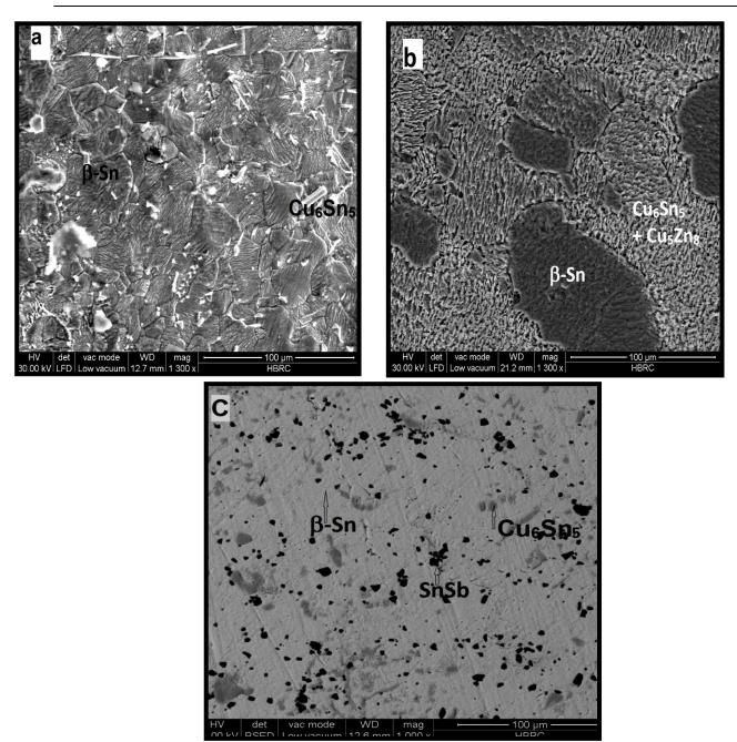
Fig. (5): Shows SEM micrographs of (a) Sn-0.7 Cu (b) Sn-0.7 Cu-2.0 Zn and (c) Sn-0.7 Cu-2.0 Sb solders
