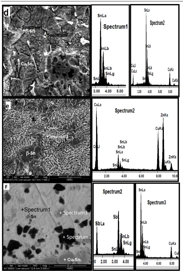
Fig. (5 d, e, f): Shows SEM, EDX micrographs of (d) Sn-0.7Cu (e) Sn-0.7 Cu-2.0 Zn and (f) Sn-0.7 Cu-2.0 Sb solders
