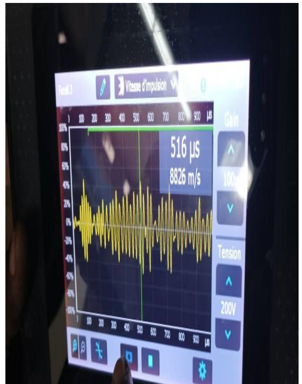
Fig. (9): Figures a) and b), respectively, show the vertical section of the Trico II and the measurement in pulse-echo mode on one grid.
