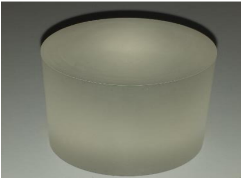
Fig. (3): A sapphire filter segment that is 5 cm in length with a 5cm diameter
