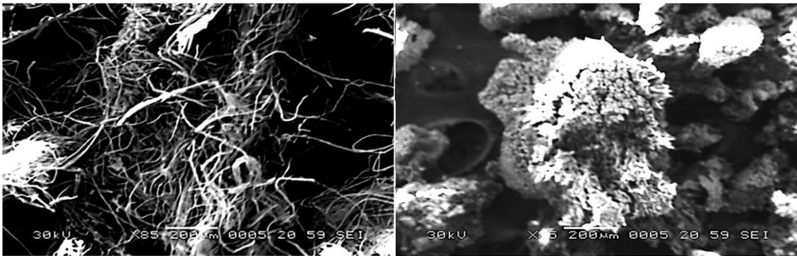
Fig. (4): SEM images of the synthesized MCC (left) and SPS (right) (magnification 85x)
