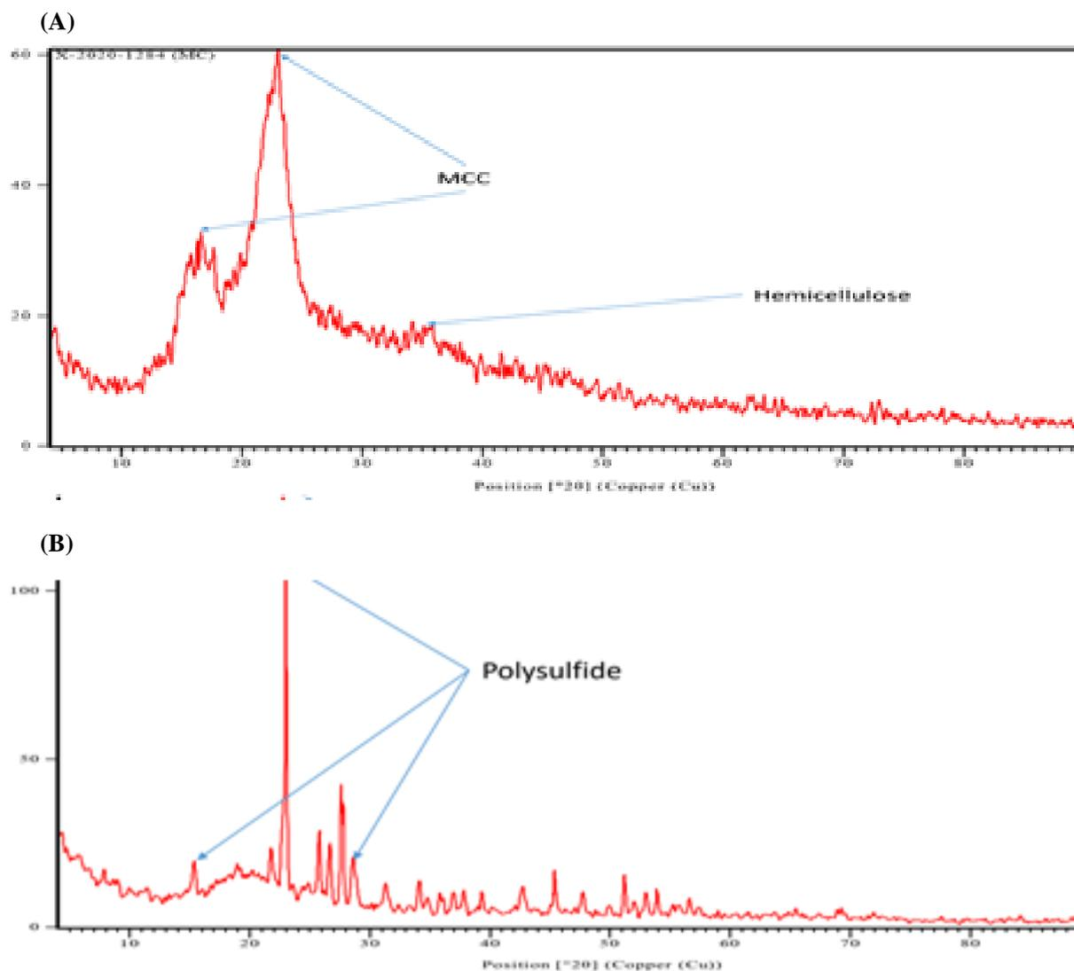
**Fig. (2): XRD characterization (degree of crystallization) of (A) MCC and (B) SPS**
