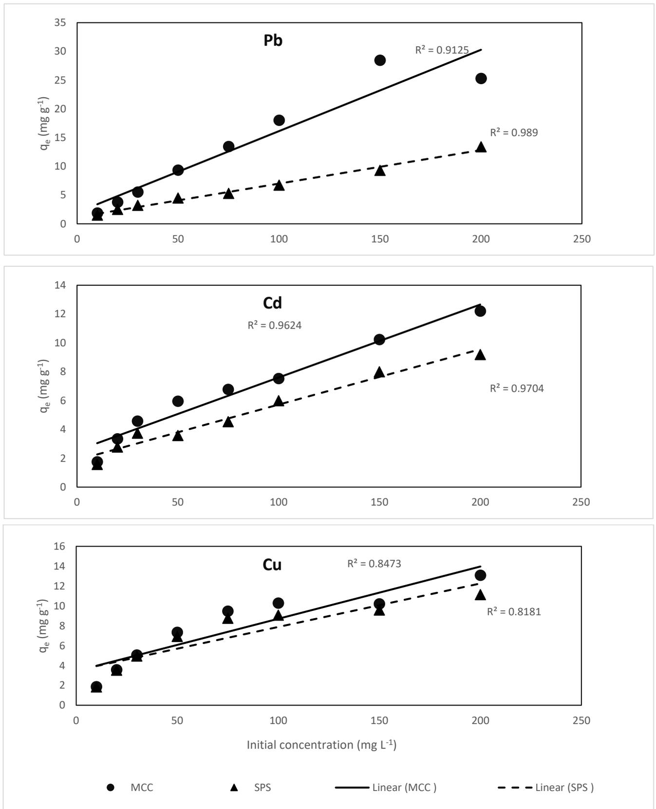
**Fig. (11): Effect of solution initial concentration (mg L<sup>-1</sup>) on sorbed amounts (mg g<sup>-1</sup>) of PTEs (Pb, Cd and Cu) from their aqueous Solutions using sorbent materials**
