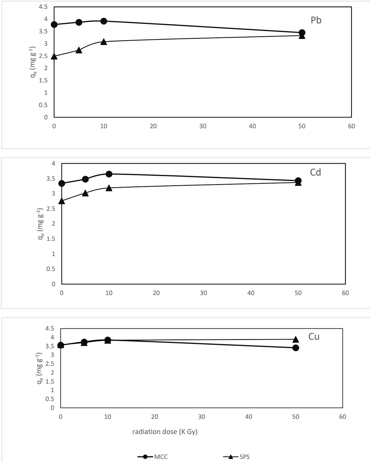
**Fig. (12): Effect of Radiation Dose (K Gy) on sorption amount ( $\text{mg g}^{-1}$ ) of water contaminants (Pb, Cd, and Cu) from their aqueous solutions using sorbent materials**
