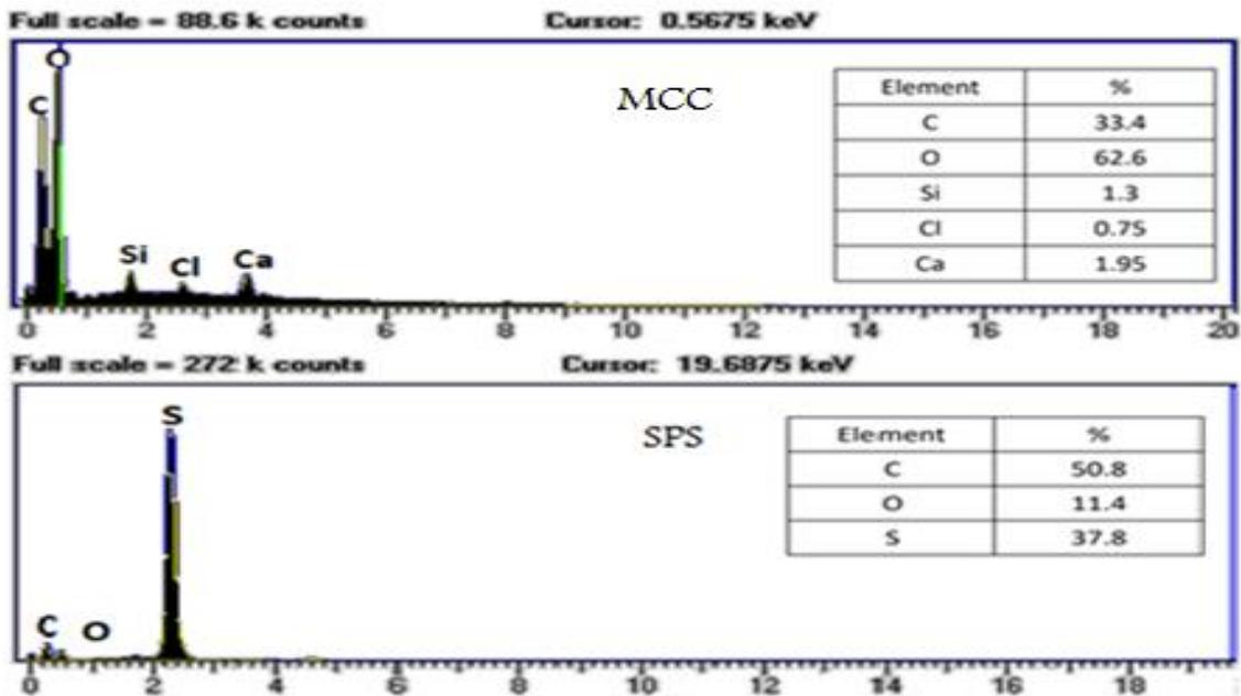
Fig. (3): EDX analysis (% of elementary analysis) for the synthesized MCC and SPS
