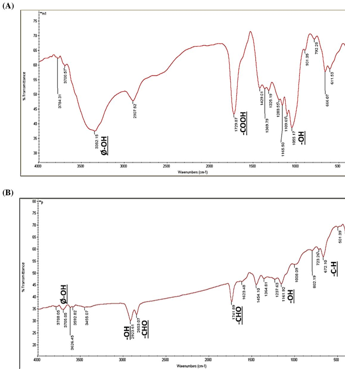
**Fig. (1): FT-IR characterization of (A) :MCC and (B): SPS for functional groups**
