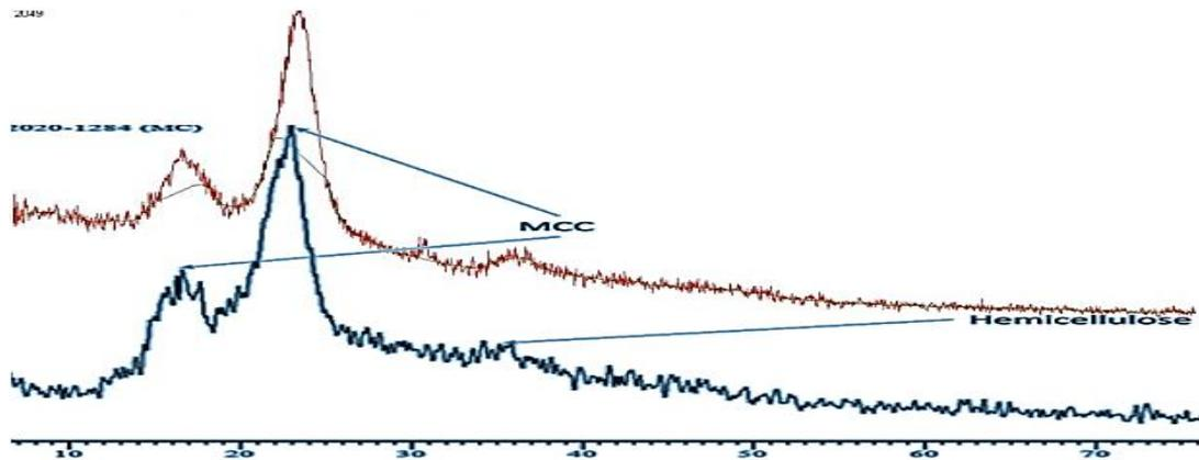
Fig. (9): XRD analysis for MCC and M-10
