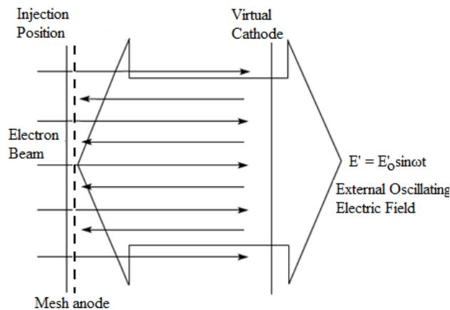
Figure (1) Simple model of axial vircator mechanism
