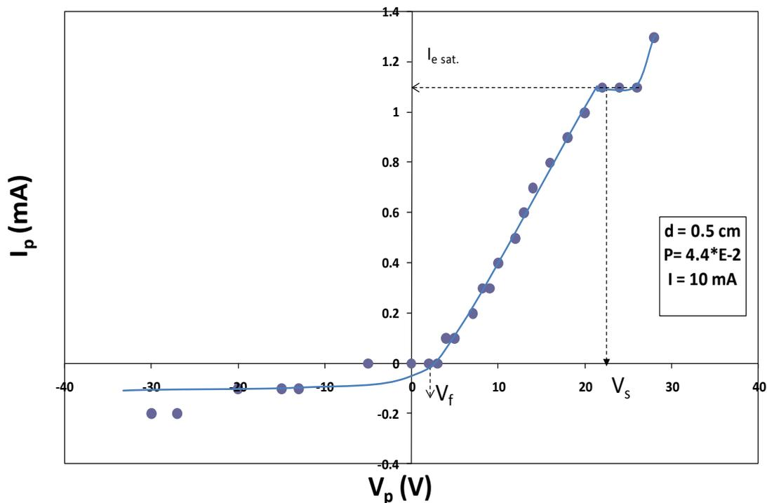
Figure (5) Characteristic curve of the electric probe
