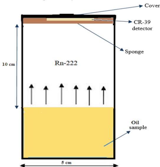
**Fig. (1): Sealed-can technique of radon measurements**
