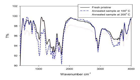
Fig. (6.b): FTIR spectrum of fresh pristine and annealed fresh samples at 100 and 200  $^\circ\mathrm{C}$
