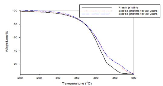
Figure (3): Thermogravimetric analysis for pristine fresh sample and pristine stored samples for 20 and 30 years ago
