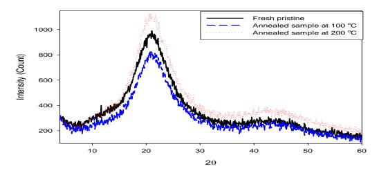
Fig. (5.a): The X-ray diffraction spectrum of pristine and annealed fresh samples
