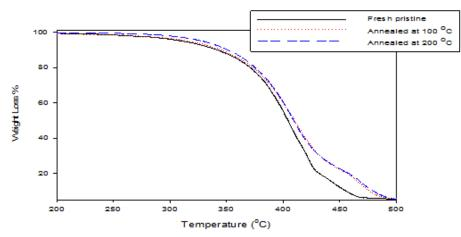
Figure (2.a): The rmogravimetric analysis for pristine and heated treatment fresh samples
