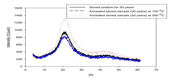
Fig. (5.b): The X-ray diffraction spectrum of stored sample for 20 years and annealed samples
