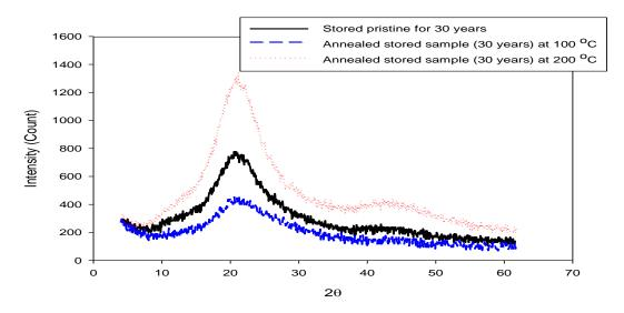
Fig. (5.c): The X-ray diffraction spectrum of stored sample for 30 years and annealed samples.
