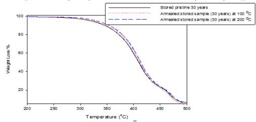
Figure (2.c): Thermogravimetric analysis for pristine and heated treatment samples stored for 30 years ago
