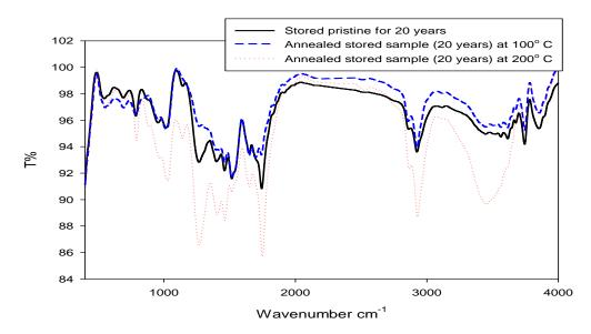
Figure (6.c): FTIR spectrum of stored pristine for 20 years and annealed stored samples at 100 and 200°C
