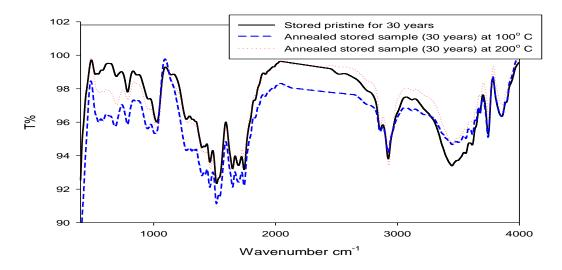
Fig. (6.d): FTIR spectrum of stored pristine for 30 years and annealed stored samples at 100 and  $200^\circ\mathrm{C}$
