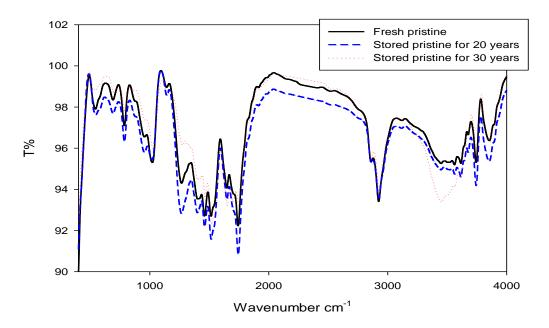
Fig. (6.a): FTIR spectrum of fresh pristine and stored pristine for (20 and 30) years
