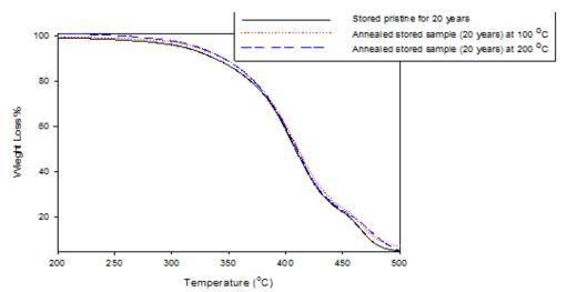
Figure (2.b): Thermogravimetric analysis for pristine and heated treatment stored samples for 20 years ago
