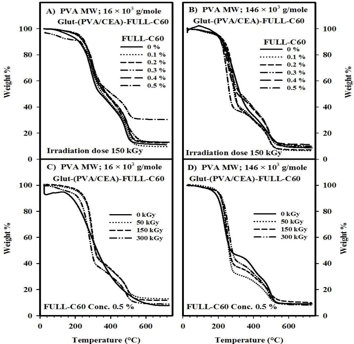
Figure (4): TGA thermograms of glutaraldehyde crosslinked of A) PVA molecular weights  $16 \times 10^3$  g/mole Glut-(PVA/CEA)-FULL-C60, (B) PVA molecular weights  $146 \times 10^3$  g/mole Glut-(PVA/CEA)-Full-C60, Full-C60 concentration 0.5 %, irradiated at absorbed doses up to 300 kGy
