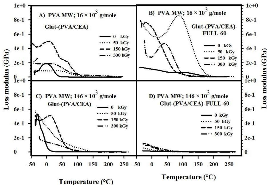
**Figure (7): Loss modulus of FULL-60 concentration 0.5 % as a function of absorbed dose up to 300 kGy. (A): Blank Glut-(PVA-CEA) of PVA molecular weights  $16 \times 10^3$  g/mole, (B): Glut-(PVA/CEA)-FULL-C60 of PVA molecular weights**
