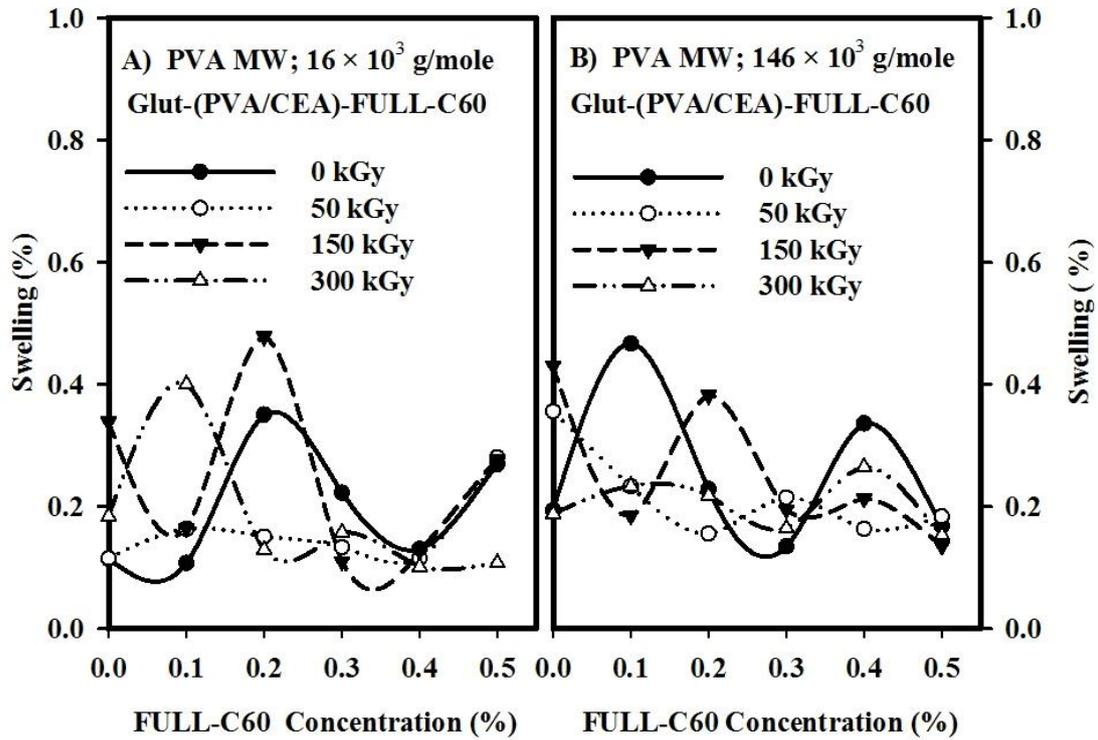
Figure (2): Degree of swelling of glutaraldehyde crosslinked of A) PVA molecular weights  $16 \times 10^3$  g/mole Glut-(PVA/CEA)-FULL-C60, (B) PVA molecular weights  $146 \times 10^3$  g/mole Glut-(PVA/CEA)-FULL-C60, as a function of irradiation dose and FULL-C60 content
