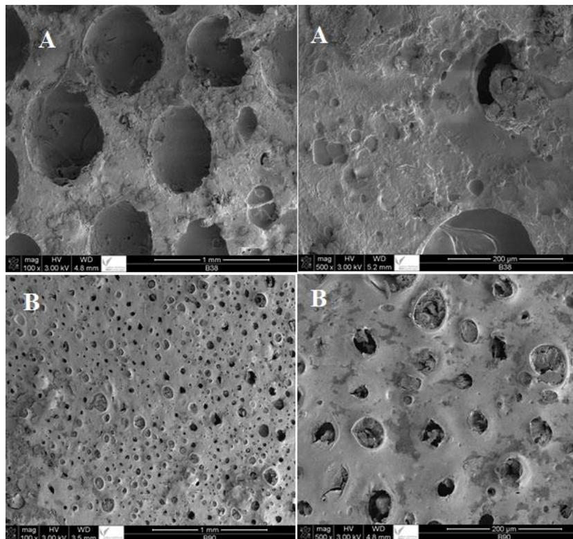
Figure (3): SEM micrographs of glutaraldehyde crosslinked of A) PVA molecular weights  $16 \times 10^3$  g/mole Glut-(PVA/CEA)-FULL-C60, (B) PVA molecular weights  $146 \times 10^3$  g/mole Glut-(PVA/CEA)-FULL-C60, FULL-C60 concentration 0.1 %, irradiated to absorbed doses of 150 kGy
