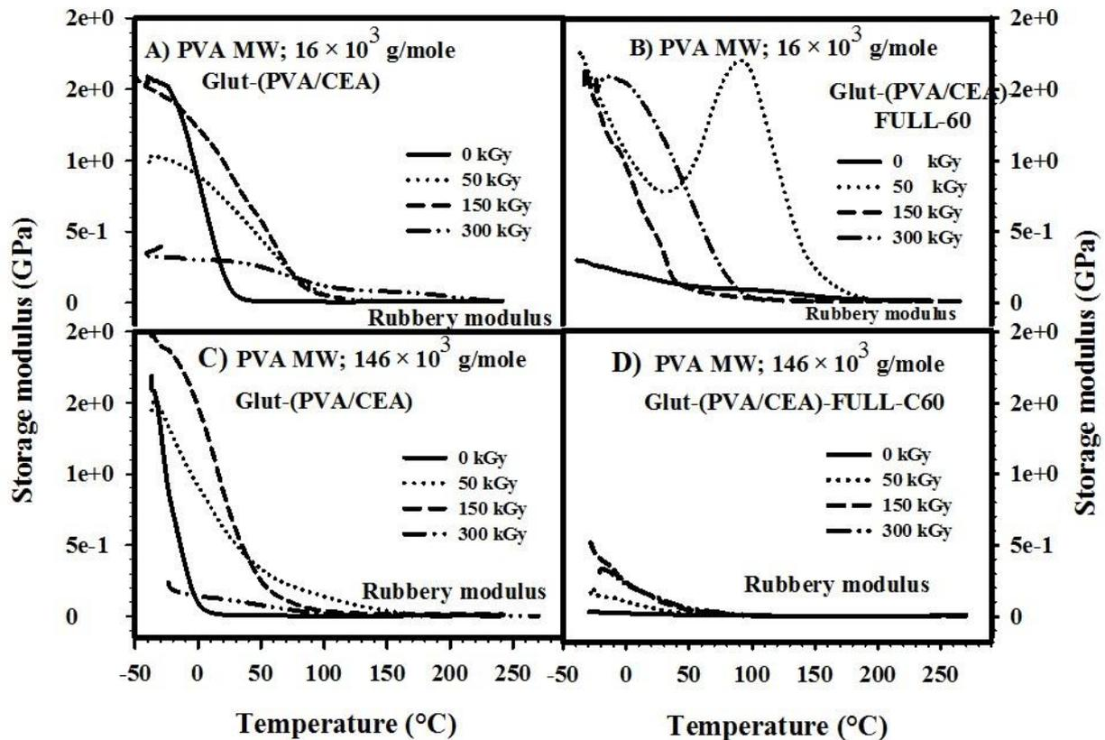
Figure (6): Storage and rubbery moduli of FULL-60 concentration 0.5 % as a function of absorbed dose up to 300 kGy. (A): Blank Glut-(PVA-CEA) of PVA molecular weights  $16 \times 10^3$  g/mole (B): Glut-(PVA/CEA)-FULL-C60 of PVA molecular weights  $16 \times 10^3$  g/mole (C): Blank Glut-(PVA-CEA) of PVA molecular weights  $146 \times 10^3$  g/mole and (D): Glut-(PVA/CEA)-FULL-C60 of PVA molecular weights  $146 \times 10^3$  g/mole
