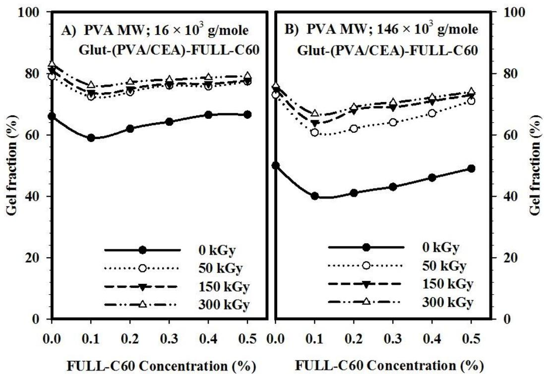
Figure (1): Gel fraction (%) of glutaraldehyde crosslinked of A) PVA molecular weights  $16 \times 10^3$  g/mole Glut-(PVA/CEA)-FULL-C60, (B) PVA molecular weights  $146 \times 10^3$  g/mole Glut-(PVA/CEA)-FULL-C60, as a function of irradiation dose and FULL-C60 content
