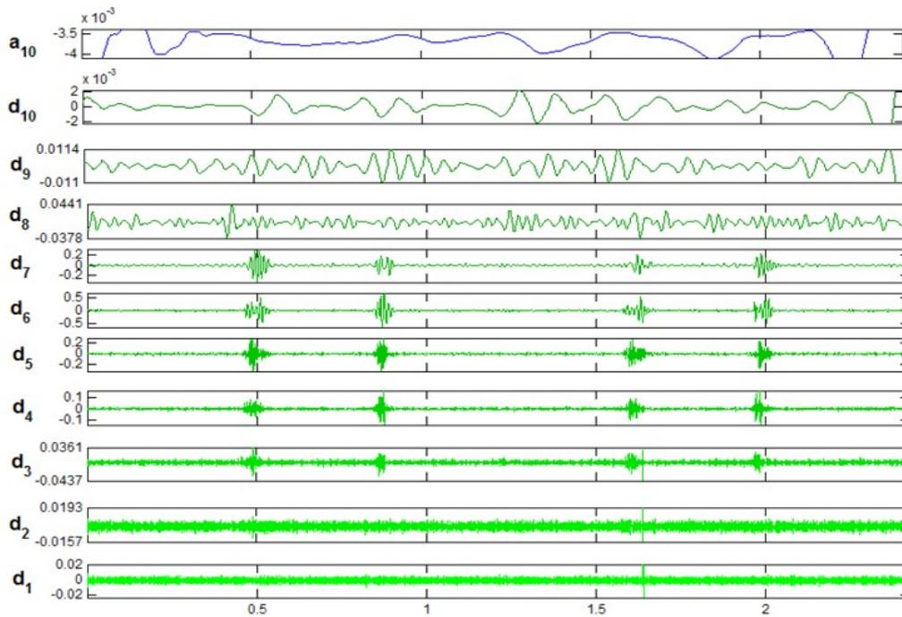
Fig. (7): Wavelet Coefficients for normal sound signal at tenth level of decomposition
