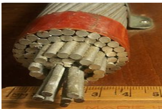
Fig. (1): Aluminum Cored Steel Reinforced (ACSR)
