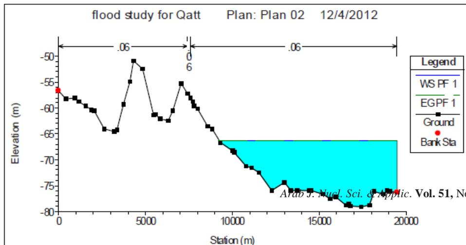
Fig. (4) Geometry of a cross section in study area
