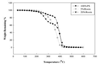
Fig. (5): TGA thermogram of PS and its blends (PS/ rosin) at various compositions irradiated at 100 kGy
