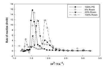
Fig. (7): Rate of reaction (dw/dt) of unirradiated PS and its blends (PS/ rosin) at various compositions
