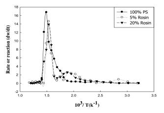
Fig. (9): Rate of reaction (dw/dt) of PS and its blends (PS/ rosin) at various compositions irradiated at 200 kGy
