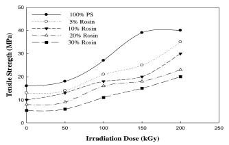
Fig. (2): Effect of irradiation dose on the Ts of PS and its blends (PS/ rosin) at various compositions
