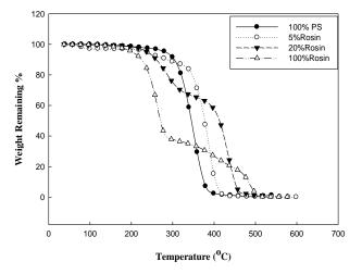
Fig. (4): TGA thermogram of unirradiated PS and its blends (PS/ rosin) at various compositions
