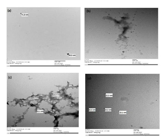
Fig. (4): TEM images of chitosan (4a), mucilage (4b), nanocomposite (4c), and irradiated chitosan (4d)
