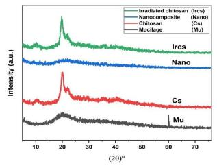
Fig. (2): XRD patterns of irradiated chitosan, nanocomposite, chitosan LMW, and mucilage
