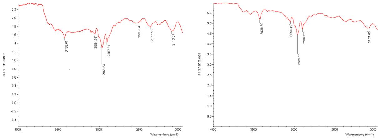
**Figure (12) Polyester samples before and after treatment by microwave radiation**
