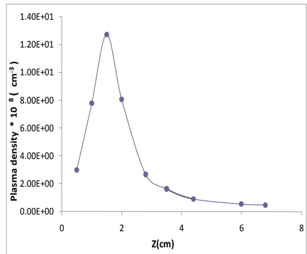
Figure (9) Axial distribution of the plasma density
