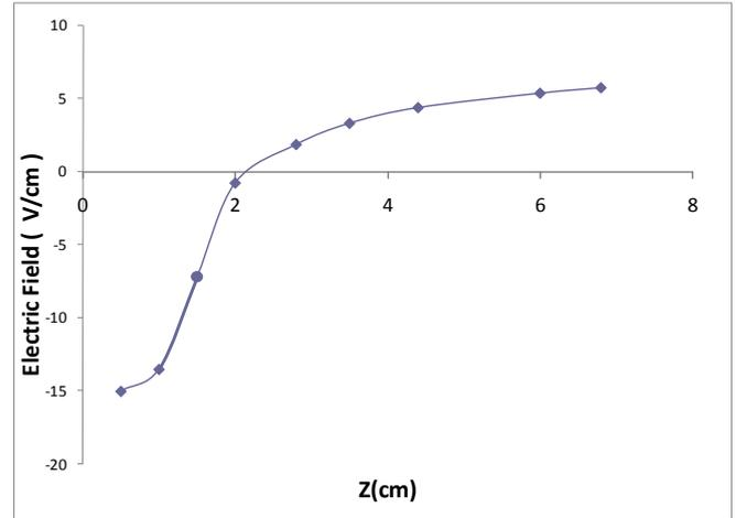
Figure (8) Axial distribution of the electric field
