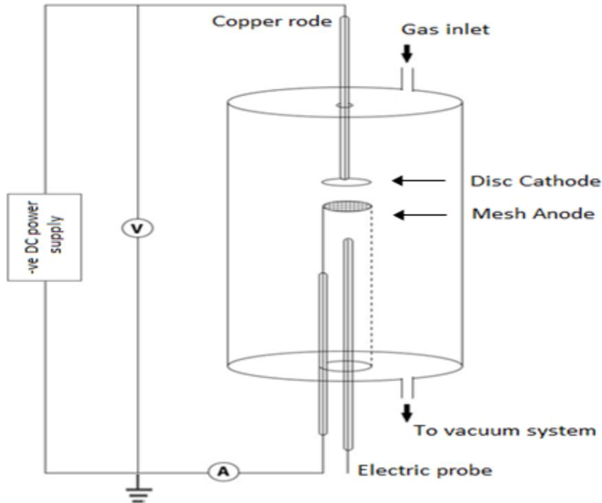
Figure (2) Schematic diagram of the system
