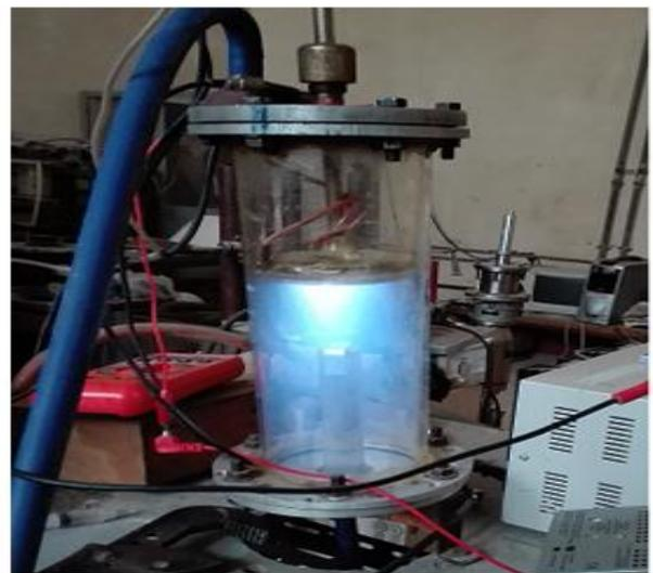
**Figure (13) Aluminum sample exposed to microwave radiation**
