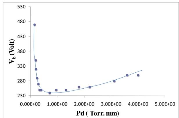
Figure (4) Paschen curve breakdown voltage  $V_b$  versus  $pd$  for Nitrogen gas
