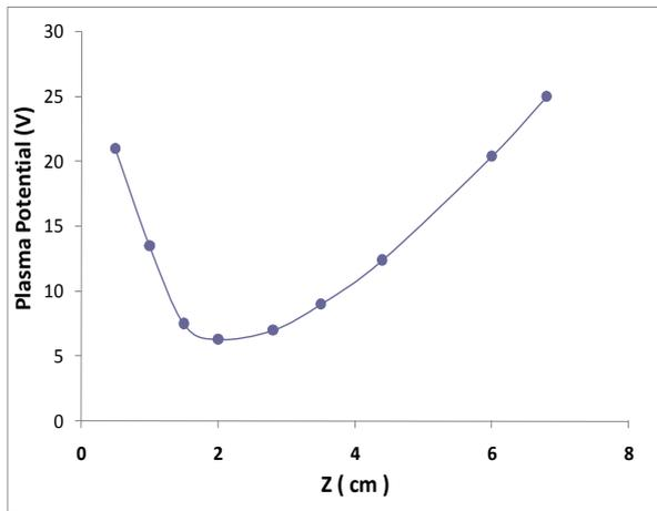
Figure (7) Axial distribution of the plasma potential
