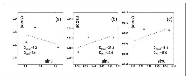
Fig. (4): W-H plots for different MgFe<sub>2</sub>O<sub>4</sub> samples
