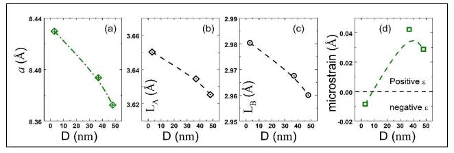
Fig. (2): a) The lattice parameter *a*, The hopping lengths b) L<sub>A</sub> for the tetrahedral site, c) L<sub>B</sub> for the octahedral site,
