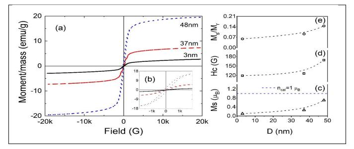
Fig. (8): a,b) Room temperature hysteresis loops, c) The observed saturation magnetization (M<sub>obs</sub>), d) coercivity (H<sub>c</sub>), and e) the squareness ratio (R<sup>2</sup>=M<sub>r</sub>/M<sub>s</sub>)
