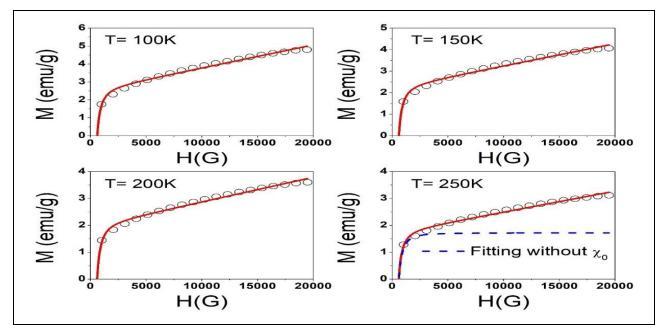
Fig. (12): The fitting of M(H) of MF1 sample with D=3nm at different temperatures according to Eq. (18)
