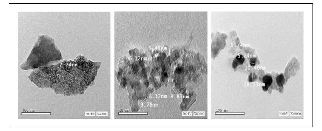
Fig. (5): TEM images of different MgFe<sub>2</sub>O<sub>4</sub> samples
