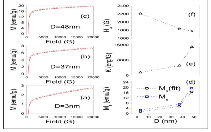
Fig. (9): a,b,c) The fitting of room temperature of M(H) according to Eq. (18), d) Ms and Ms(fit), e) effective magnetic anisotropy constant (K), and f) the anisotropy field (H<sub>a</sub>) for different MgFe<sub>2</sub>O<sub>4</sub> samples
