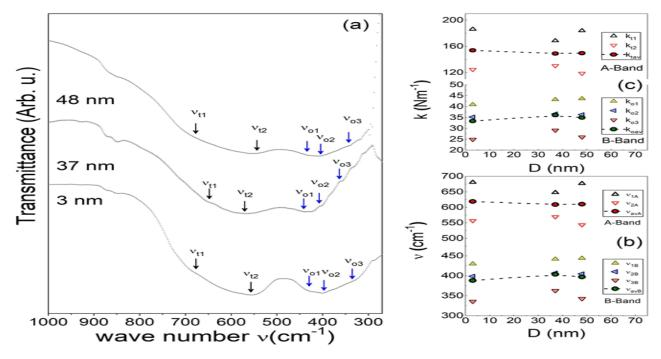
Fig. (6): a) FTIR spectra, b) vibrational frequencies (v), and c) force constants (k) for different MgFe<sub>2</sub>O<sub>4</sub> nanoparticles
