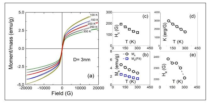
Fig. (11): a) Hysteresis loops at different temperatures, b) M<sub>s</sub>, and M<sub>s</sub> (Fit), c) coercivity (H<sub>c</sub>), d) effective magnetic anisotropy constant (K), and e) the anisotropy field (H<sub>a</sub>) for different MgFe<sub>2</sub>O<sub>4</sub> samples
