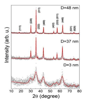
Fig. (1): XRD patterns of different MgFe<sub>2</sub>O<sub>4</sub> samples and the average particle size (D) is indicated for each sample. Red lines represent Rietveld refinement using MAUD
