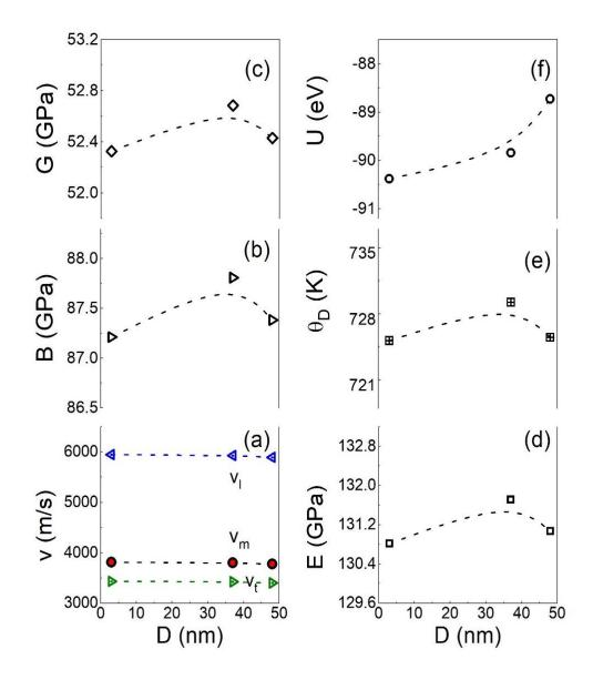
Fig (7): a) Elastic wave velocities (V<sub>1</sub>, V<sub>t</sub> and V<sub>m</sub>), elastic constants: b) Bulk modulus B, c) rigidity modulus G, and d) Young's modulus E, e) the Debye temperature (θ<sub>D</sub>), and f) the lattice energy (U) for different MgFe<sub>2</sub>O<sub>4</sub> samples
