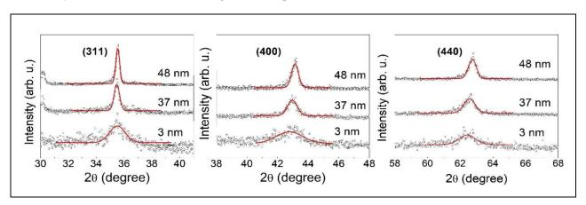
Fig. (3): Gaussian fitting of (311), (400), and (440) XRD peaks for different MgFe<sub>2</sub>O<sub>4</sub> nanoparticles
