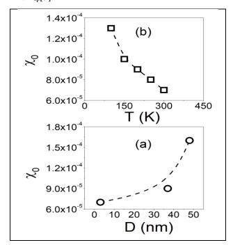
Fig. (10): The dependence of linear contribution of the magnetization (χ<sub>0</sub>) on: a) The particle size at 300K, and b) temperature for the sample MF1 (3nm)
