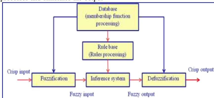
Figure (1): Main structure of fuzzy inference system
